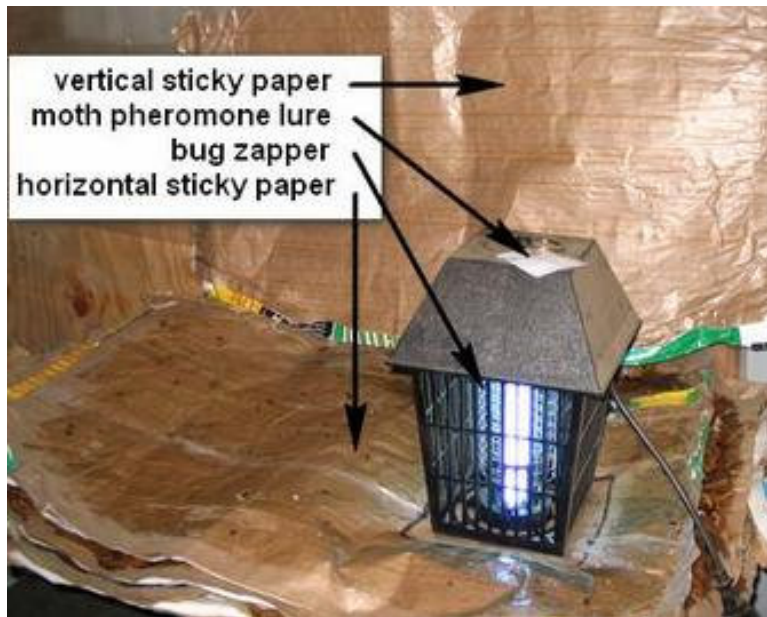
Bug zapper with pheromone and sticky paper. Horizontal sticky paper was effective but vertical sticky paper was not effective.
