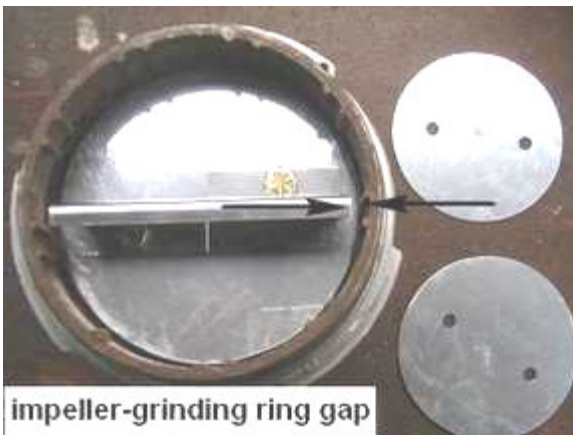
Figure 8. Hulling gap is the distance between impeller blade and grinding ring.
