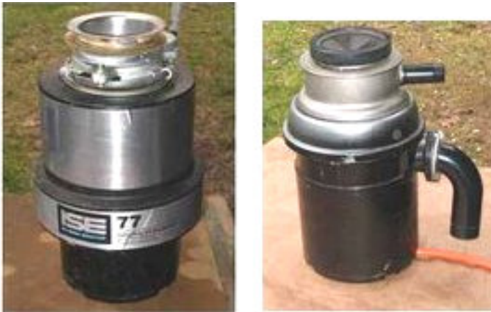
Figure 1. Kitchen sink garbage disposer, ISE 77, equivalent to Sears Kenmore 700, \frac{3}{4} horsepower disposer (left) and converted centrifugal impact huller (right).
