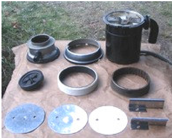
Figure 5. Components for converting the garbage disposer into grain huller: Top row, left to right, hopper, hopper retaining ring and garbage disposer motor. Middle row, rubber splash guard, rubber faced ring and the steel grinding ring. Bottom row: 3 turntable disks (5, 5 1/8 and 5 1/4 inch diameters) and 2 impeller blades (4 1/2 and 4 3/4 inch long).
