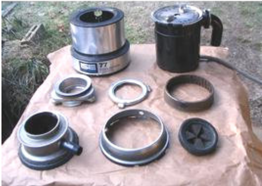
Figure 2. Disassembled garbage disposer: top row, left to right: insulated jacket and motor. Middle row, sink flange, sink mounting ring and grinding ring. Bottom row: hopper, hopper retaining ring and rubber splash guard.
