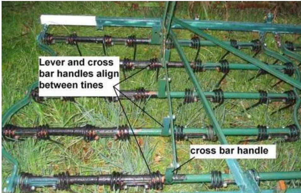
Figure 6. Lever mechanism aligned between spring harrow teeth.
