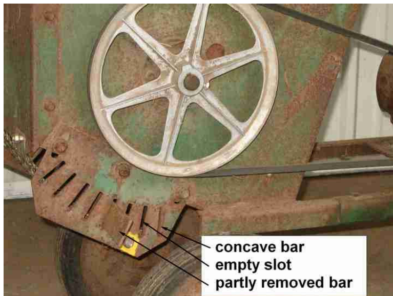
Figure 3. Close-up of concave bar, partly removed bar and empty slots.
