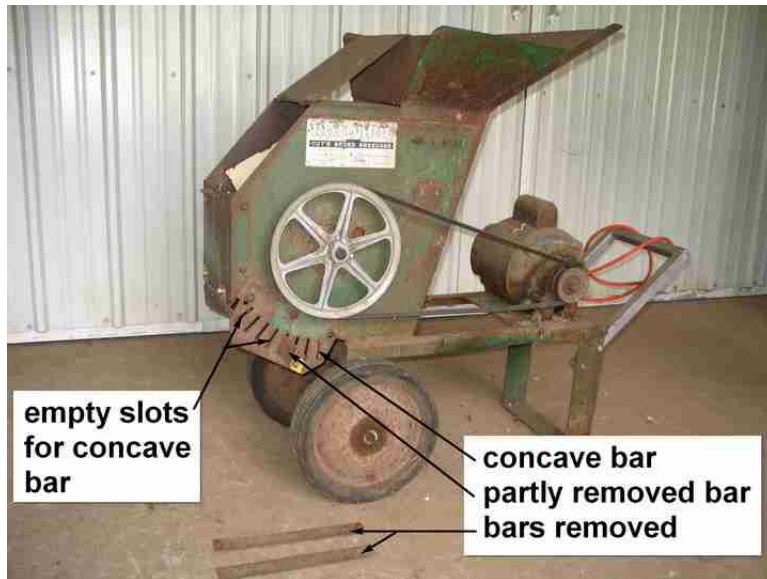
Figure 2. Converted Roto Hoe grain thresher with a 3/4 hp electric motor, 3 inch drive sheave, 10 inch hammer sheave, and concave bars.
