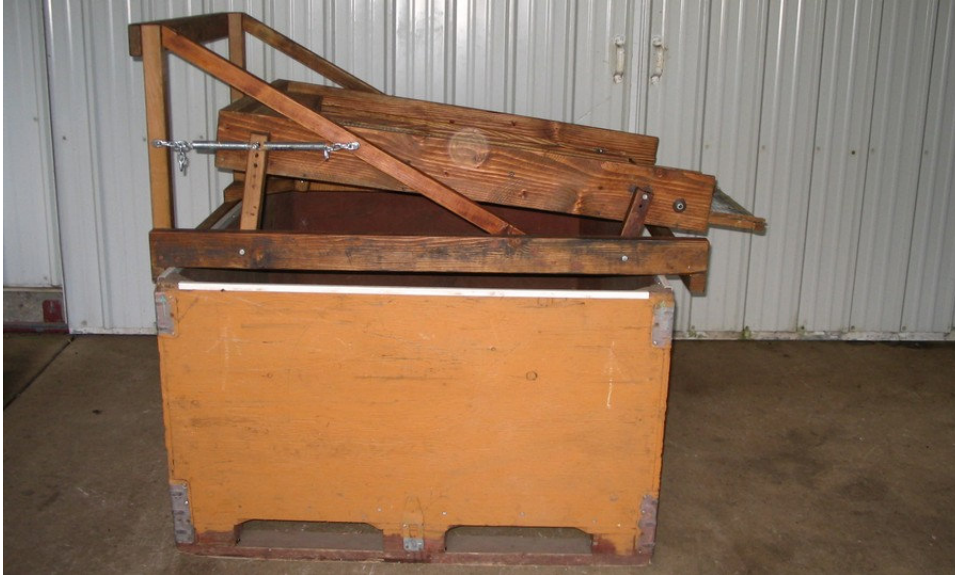
Figure 6. Hand operated screen seed cleaner elevated on a tote bin to collect seeds that pass through the screen.
