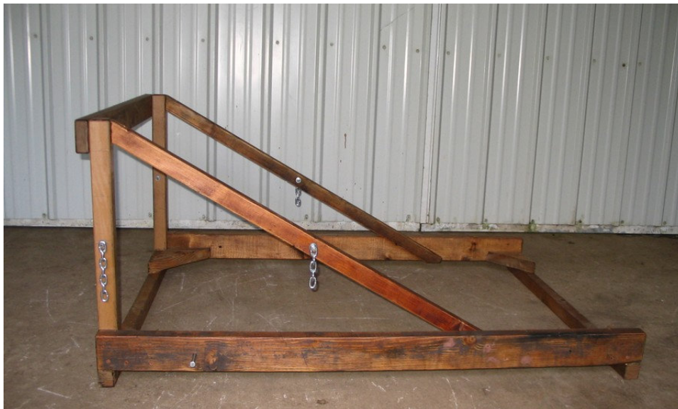
Figure 3. Frame with chains to adjust spring tension.
